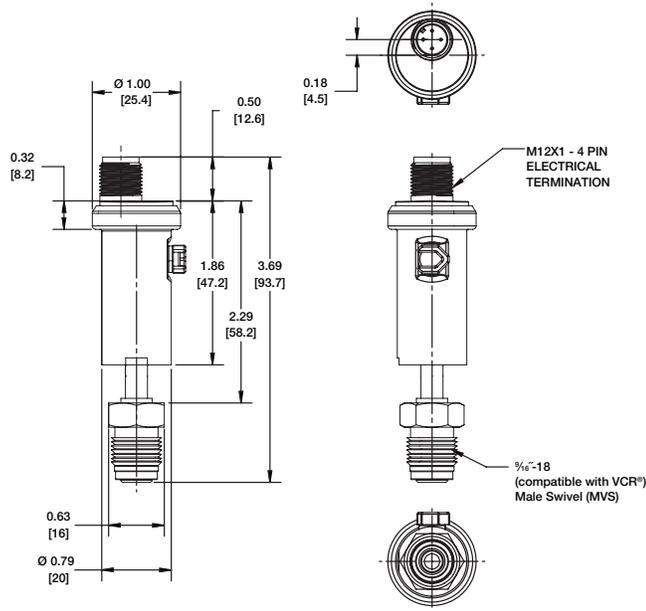
**MVT - 1/16"-18 UNF (compatible with 1/4 VCR®) Male Flow Through**
