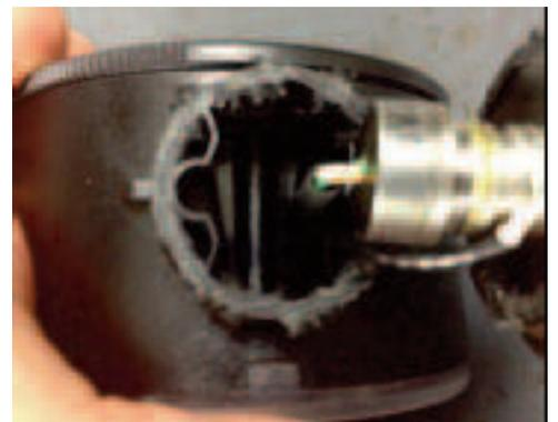
**Conclusion:** This test confirms that the DG25 enclosure is compliant with the IP-67 standard. The DG25 gauge can therefore be claimed as an IP-67 rated product.
