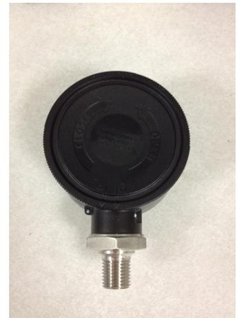
**Procedure:** Secure the test unit to a tether in order to submerge and retrieve it (in this case the unit was threaded onto a fitting, which was attached to a long length of plastic tubing). Submerge the unit in 1 meter of water for 30 minutes.
