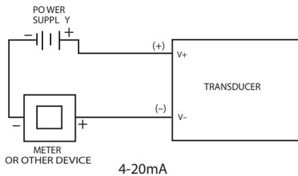
**A4 transducer has internal transient protection: for safety, limit line-to-ground voltage to 36 Vdc max.**
