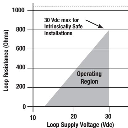
$$V_{min} = 12V + (.022A \times RL) \text{ (includes a 10\% safety factor)}$$
