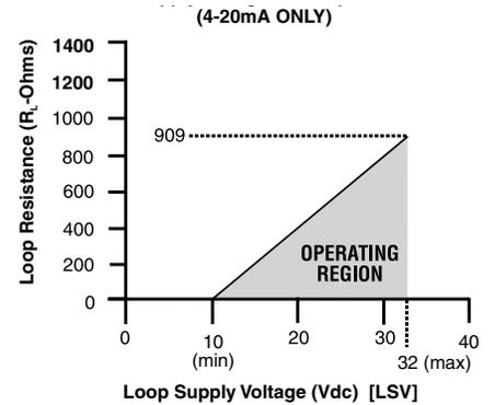
To determine minimum loop supply voltage:
