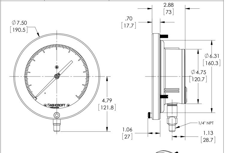
Note: 3 Mounting studs threaded equally spaced on a 7" [178] Bolt Circle.
