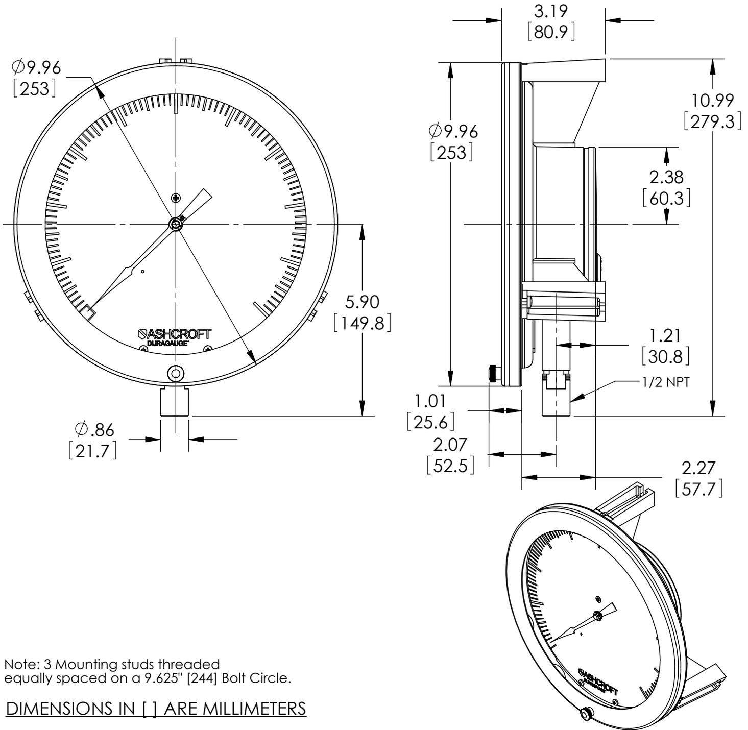
Note: 3 Mounting studs threaded equally spaced on a 9.625" [244] Bolt Circle.
