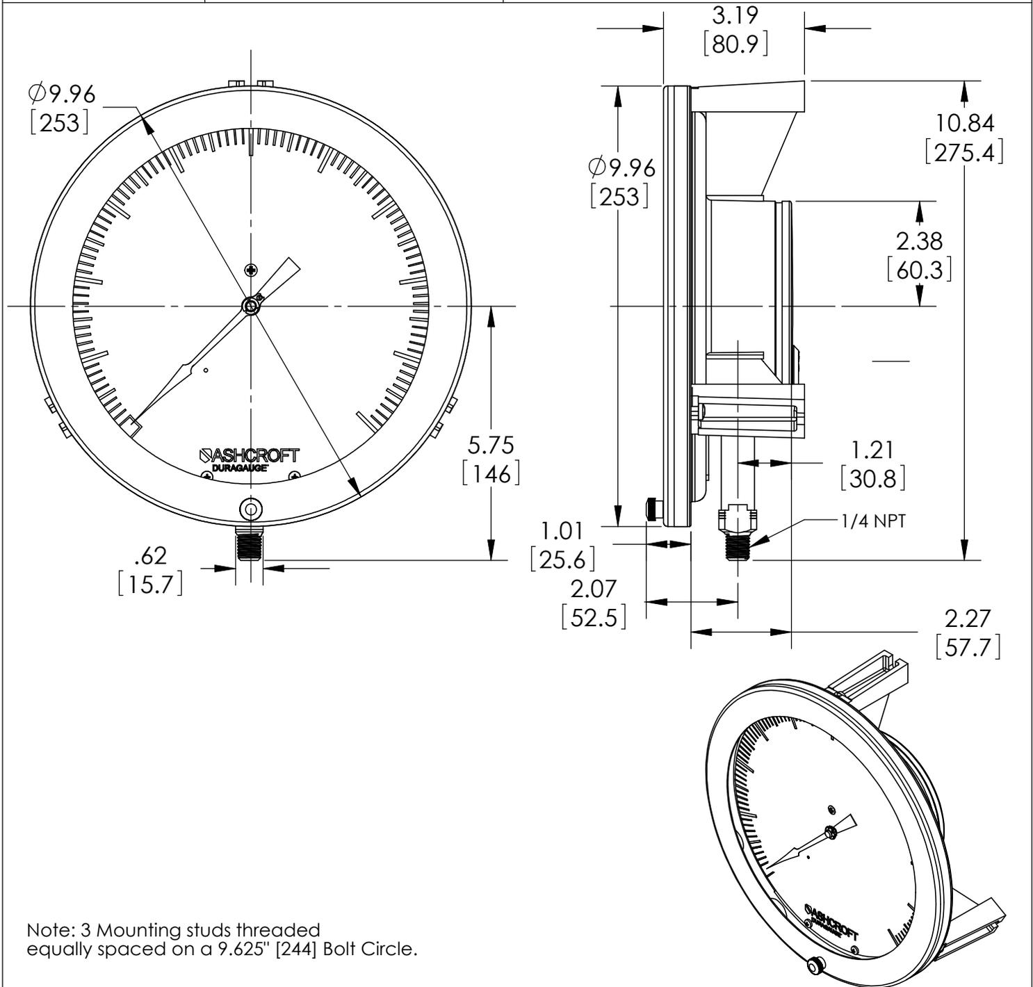
Note: 3 Mounting studs threaded equally spaced on a 9.625" [244] Bolt Circle.
