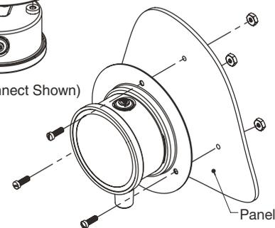
NOTE: Use an open end wrench on the gauge process connection when connecting gauge to pressure source.
