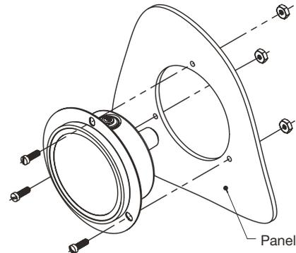
NOTE: Use an open end wrench on the gauge process connection when connecting gauge to pressure source.
