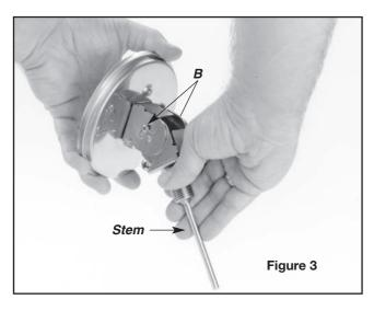
**CAUTION:** To assure longest life, the "EVERY- ANGLE" joint should be operated only when necessary during installation or removal of the thermometer.
